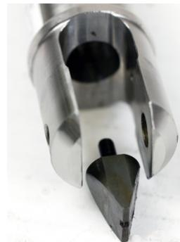
Secure the tool body in a vise (jaw end pointed down) using smooth vise jaw pad to prevent damage to the tool.
