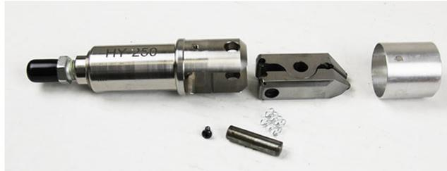
Check the rear jaw rollers and front carbide rollers for excessive wear or chipping. Replace if necessary.
