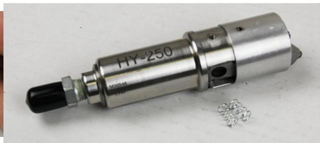
With the jaw guard and springs removed, simply push the center pivot pin out of the jaw body. The pinch off jaws can now be removed.
