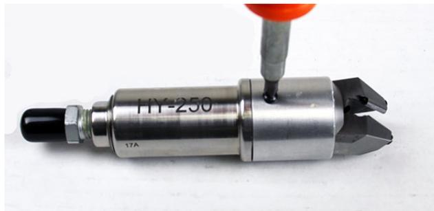
Manually manipulate the jaws by hand to the FULLY CLOSED position and “slowly” slide the jaw guard off the tool body. **NOTE: There are 2 small coil springs inside the shroud. By holding the jaws closed, the spring remains compressed during this disassembly and will prevent the springs from damage. Be sure to catch the springs as they are exposed.**
