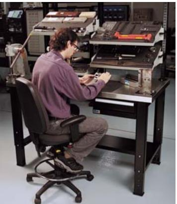
Workbenches with bolting adjustable height legs allow this avionics repair facility to adjust the workbench height as personnel and usage change over time.
