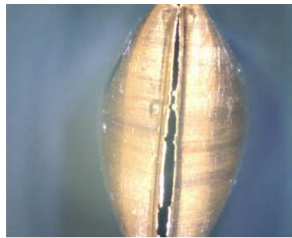
Example of tubing that was too hard and separated prematurely during the pinch-off process.
