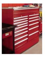
Lista created a custom toolbox for service technicians at United Auto Group dealerships. The cabinet combination includes a Double Width cabinet mounted over two Standard Width cabinets, and a special "skirt" to hide the mobile base.
