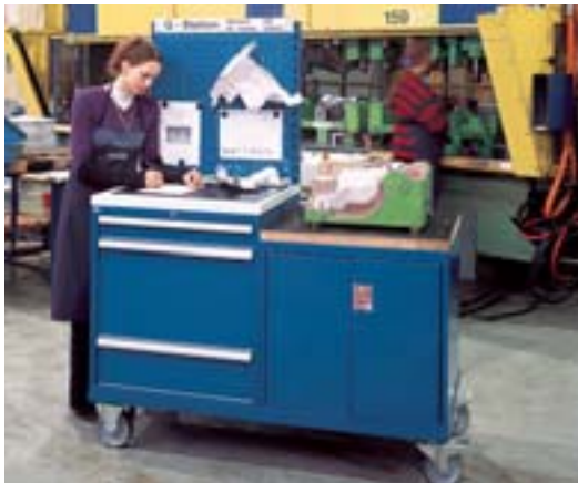
Drawer and door cabinets form a mobile workcenter that serves as a quality station.
