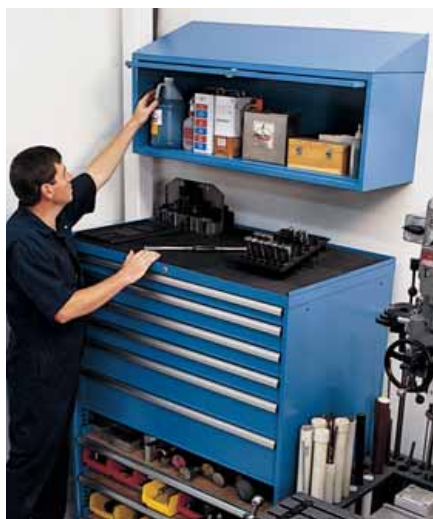
An overhead cabinet with retractable door provides convenient bulk storage above a drawer cabinet in the machining area of an aircraft repair facility.
