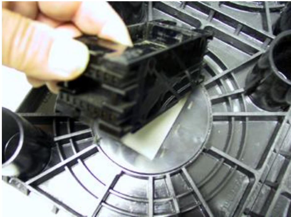
Picture 9-8 Installing Powerport Clips
