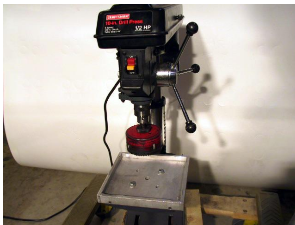
Drill Press w/ 4" hole saw
