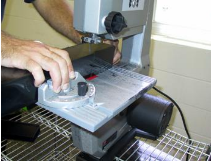
Picture 7-4 Cutting Perimeter
