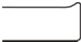
side view of solid shelf, showing raised "V" edge
